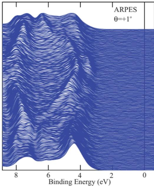
Fig.: ARPES of ZnO, source: PhD thesis of
